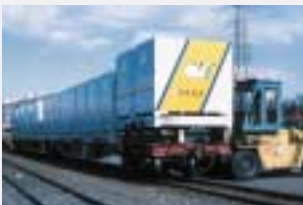
2-ton container About half as big as the usual 5-ton container, and developed to enable use of rail transport even for small cargo. Used mainly in major cities nationwide.
