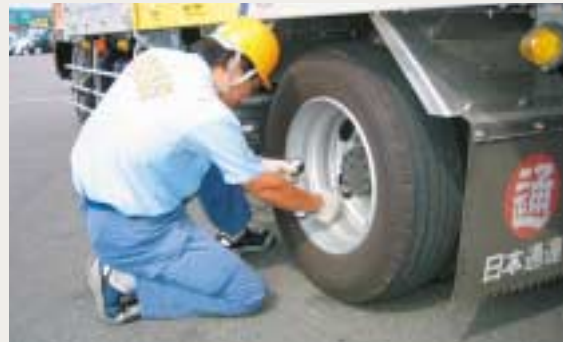
Checking air pressure of tires
