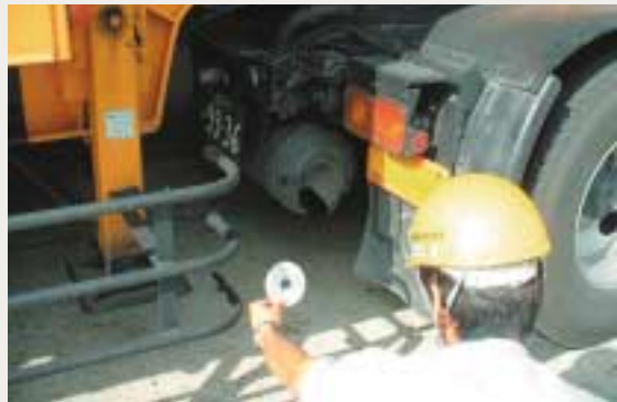
Checking black smoke (JR Container Section)
