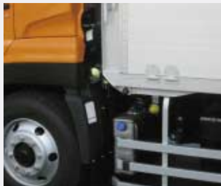
Tank with blue cap contains urea/water solution
