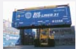
Big Ecoliner 31 Wing-door rail container with larger internal dimensions than the Ecoliner 31. Volume is that of a large truck. Useful for the modal shift from truck to rail. Used between Tokyo and Osaka and other routes.
